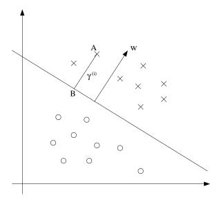
The decision boundary corresponding to (w, b) is shown, along with the vector w. Note that w is orthogonal (at 90°) to the separating hyperplane. (You should convince yourself that this must be the case.) Consider the point at A, which represents the input  $x^{(i)}$  of some training example with
